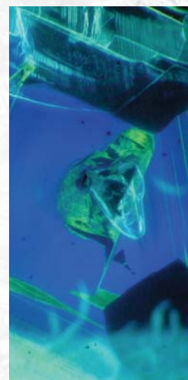
Figure 1. Cathodoluminescence image of a diamond, showing internal structure around a mineral inclusion
